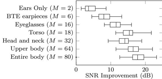
**Fig. 7:** Experimental results for MVDR beamforming on the human subject with wearable arrays having different numbers of microphones. All arrays include the reference microphones near the ear canals. The box-and-whiskers plot indicates the quartiles of the simulated SNR improvements.
