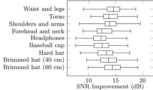
**Fig. 8:** Experimental results for MVDR beamforming on the mannequin with different microphone configurations. Each array has  $M = 18$  microphones, including the left and right reference microphones.
