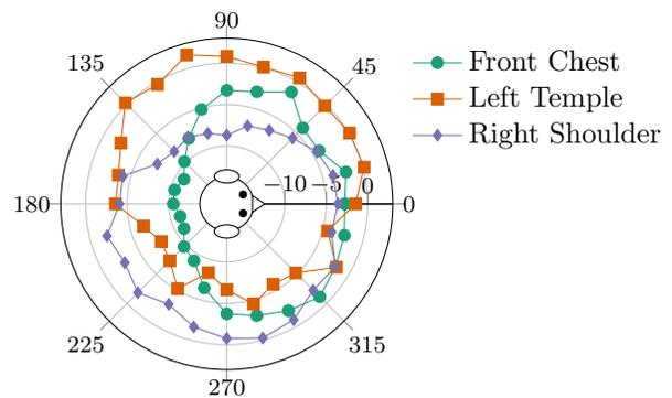
**Fig. 4:** Overall power, in dB relative to a free-space microphone, received by three microphones on the human subject.
