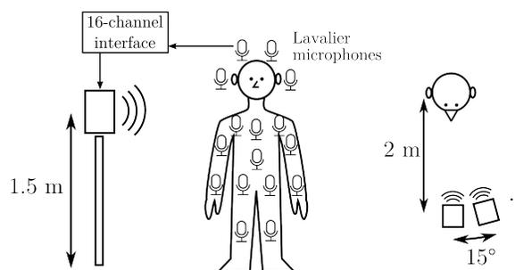
**Fig. 1:** Impulse responses were measured using a studio monitor and 16 microphones placed at 80 positions on the body and 80 positions on wearable accessories. Test signals were captured from 24 angles.
