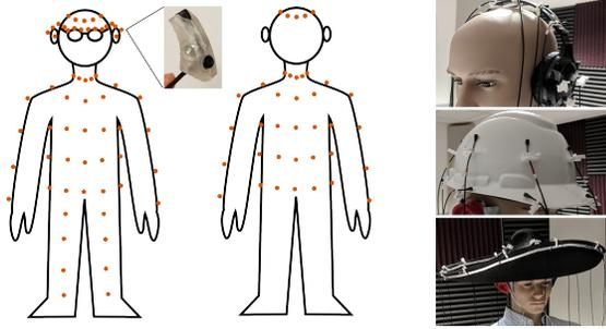
**Fig. 2:** Left: Impulse responses were measured at 80 positions on the body, including one microphone affixed to each ear and four in behind-the-ear shells. Right: Wearable accessories with 16 microphones.
